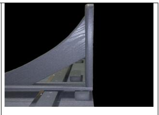
3. Mount table with corbels attached to spa just under spa shell lip using 2" screws. The number of corbels will depend on the width of the table. There will be at least 2 corbels. Tables with a cutout for a cover lifter may require a table leg to support the rear of the table.
