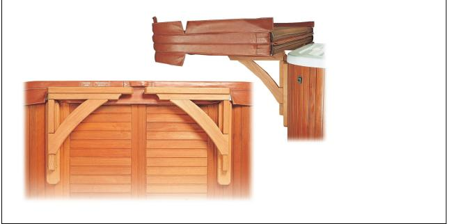
Position the Easy Slider arms as shown in the photograph above, so that the top of the arm is level with the top of the spa. Center the arms right to left allowing at least 1" clearance between the arms. Fasten to the spa cabinet with 8 each 2" screws provided making sure the uprights are plumb and the top of the arms are approximately  $1/8^{th''}$  higher than the top of the spa.
