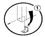
INSERT FIXED PANEL up into the middle channel of the frame at the head and lower into the THREHOLD RECESS. Slide panel as far as possible into the jamb pocket. #2
