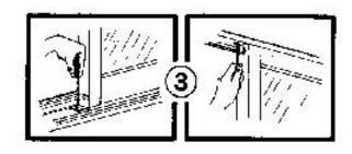
INSERT OPERATING PANEL into head and lower onto the threshold track. MAKE SURE vinyl sweeps are clear of track (Fig. 4)
